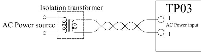
The closer the isolation transformer located to PLC input, the better. AC power wire should be twisted wire. The capacity of isolation transformer should be more than 120% consumption capacity of PLC, or the voltage at primary side of transformer would larger than rated one that will undermine safety.
