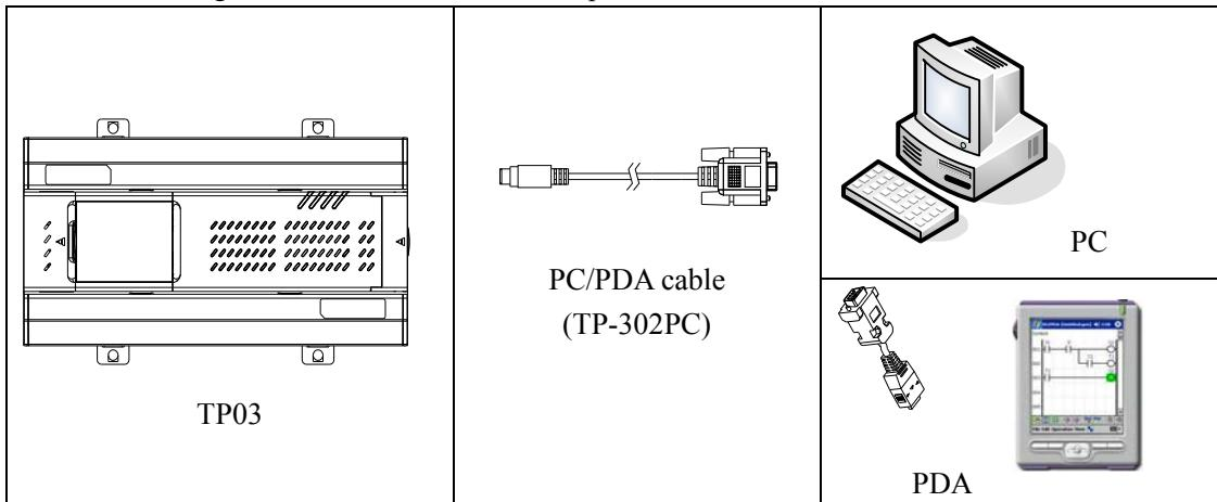
Note: User can mode the adapter that tranfers signal RS422 from 9 pin D-type connector to RS 485 on A/B terminal. Please refer to section 5 of Chapter 1 for more information about the TP-302PC Pins and its definition.
