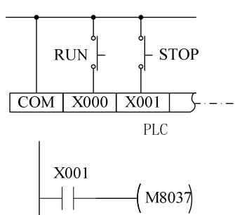
See the left figure. Please set M8035 to 1 and D8035 to 0. Then the switch for X000 and X001 can control the TP03 RUN or STOP.
