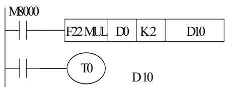
The multiplication instruction can expand the register data so the setting range will be widen. Max value should be below 32,767. In this example, D11 is automatically used by F22 MUL, do not use it at any other places.
