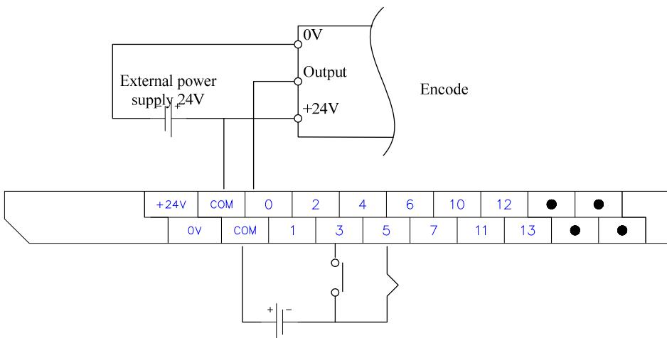
Note: All external power DC24V + terminals can be connected with the COM, while – terminal must be separated.
