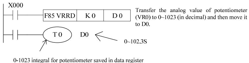
As for the above example, the input value can be multiplied with the application instruction F22.
