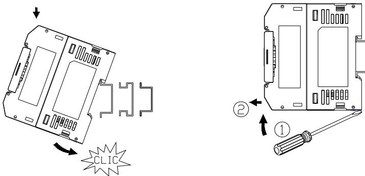
Firstly, place the groove at the back of modules right on the upper edge of Din rail. Then push the module down to lock up position.
