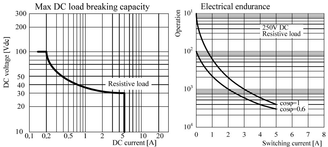
Note 1: The data in the figure are rated ones. The ambient temperature will affect the lifespan of relay.
