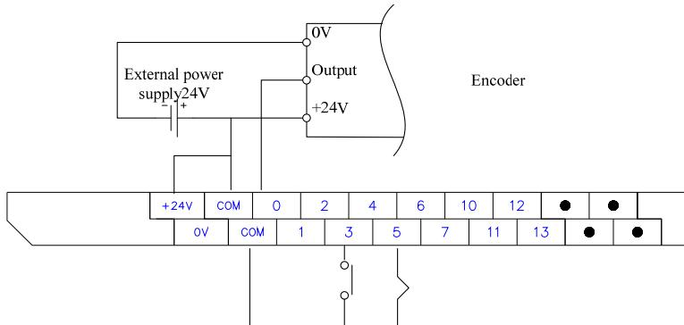
Note: External DC24V + terminal can connect with the COM on the PLC, while – terminal must be separated.
