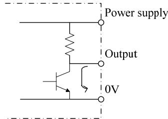
Among the above example 1, 2, 3, 4, 5, the driving current of external output transistor must be larger than that of internal transistor of input module (6~7mA).
