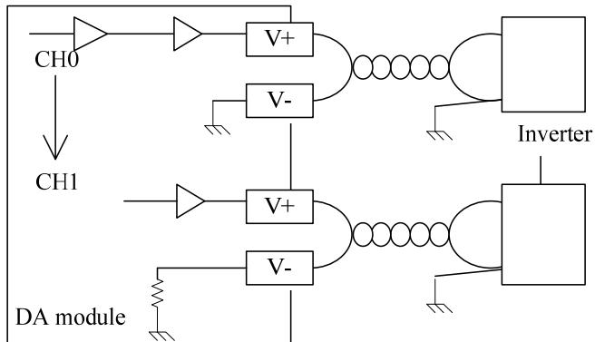
1. The cable for analog input should be standard isolated twisted cable, routed away power line and other line which will interrupt others. It is recommended that the cable should be less than 3m in length.
