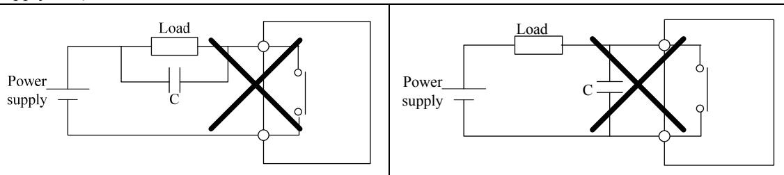
The charging current of capacitor in OFF condition is too large, so the terminal might be melt. While short circuit current of capacitor in ON condition, the terminal also might be melt out.
