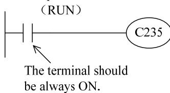
C235 is responding to X000, so X000 should not be set as the enabling terminal.
