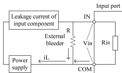
iL: leakage current
