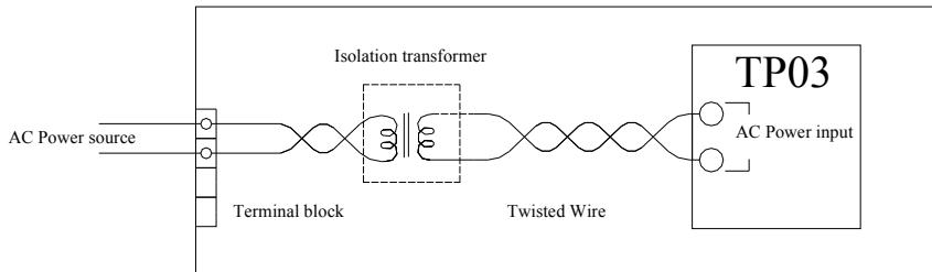
Please add a voltage tap to secondary side of transformer if the capacity of transformer is larger. The power supply for PLC should be a single one when noise is very serious. And several transformers are recommended.
