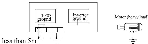
If the system can not be grounded separately, just connect the
