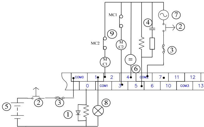
①Diode for absorbing surge: to extend the terminals lifespan.
