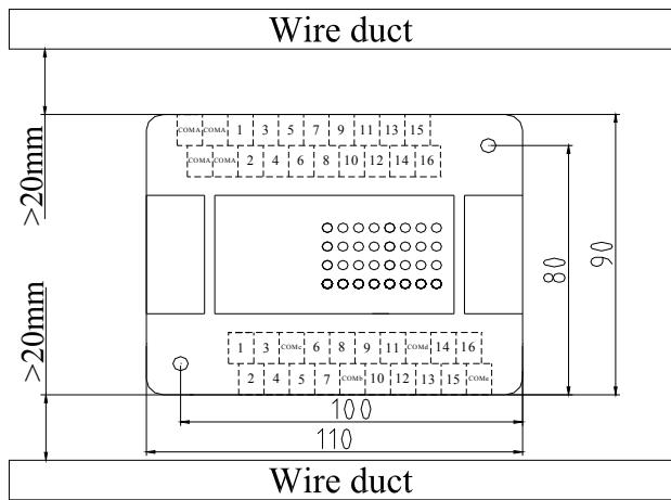
The following figure indicates dimension for installation holes when expansion cable (4cm) is used. And the fixing screw should be M4.
