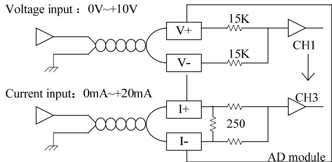
1. The cable for analog input should be standard isolated twisted cable, routed away power line and other line which will interrupt others. It is recommended that the cable should be less than 3m in length.
