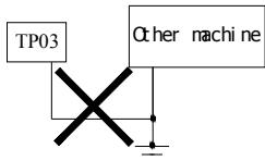
Apply Class 3 ground for TP03. The grounding wire should be  $2\text{mm}^2$  or more and less than 5 meters in length.
