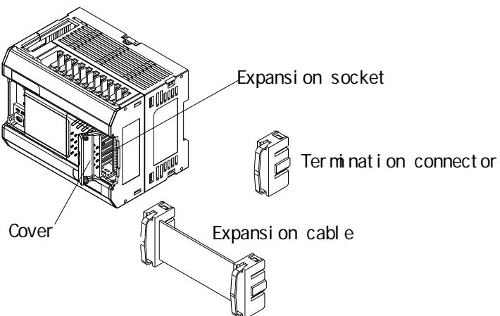
NOTE 1: Remove the expansion cable or termination connector from the expansion socket .
