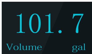
Figure 10. Display Mode 3: Remaining Volume
