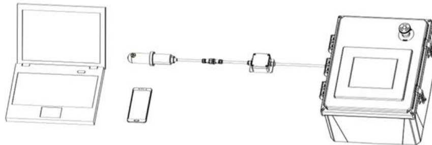
Figure 3. Bluetooth connection to ST-565 Series sensor
