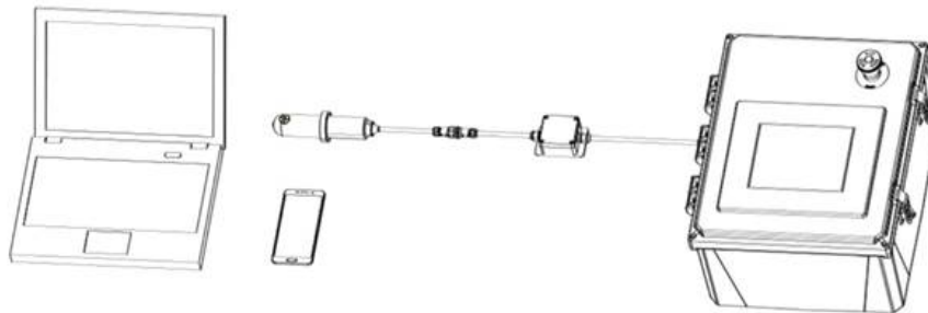
Figure 4. Bluetooth connection to ST-600 Series sensor
