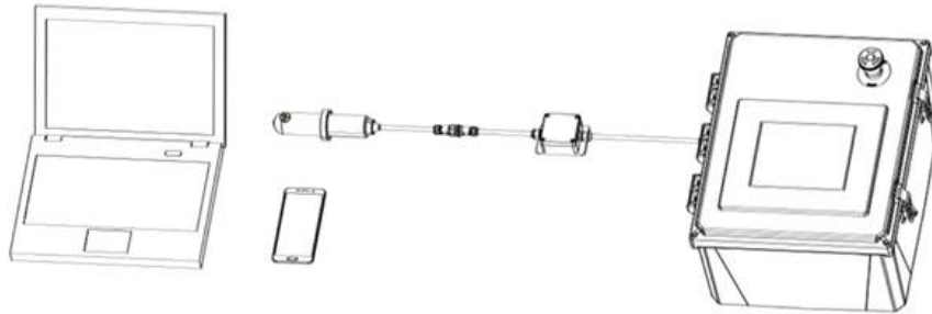
Figure 4. Bluetooth connection to EM-500 sensor
