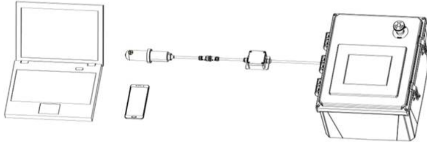
Figure 4. Bluetooth connection to ST-525 Series sensor
